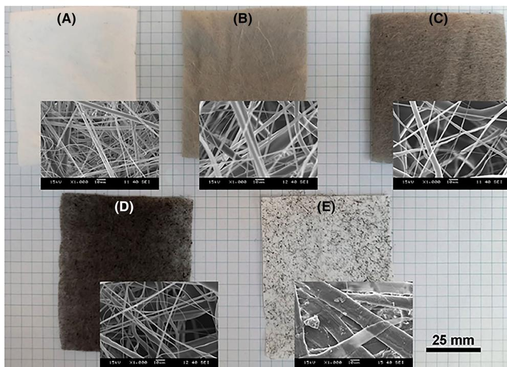
**FIGURE 3** Optical and SEM images of MB fiber mats: (A) pristine, (B) 0.1 wt% CNT, (b) 0.25 wt%, (D) 0.5 wt% CNT, and (E) 0.75 wt% CNT
