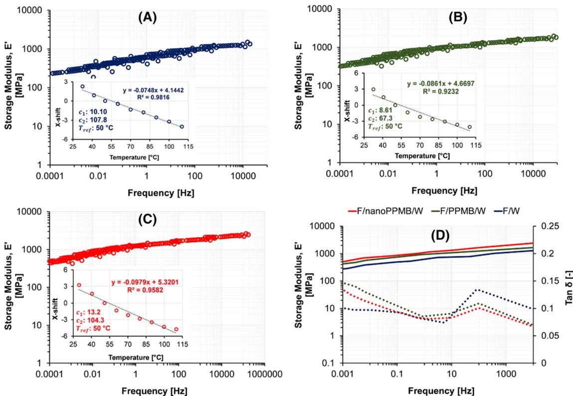
FIGURE 9 DMA curves of SPCs: Storage modulus,  $E'$ , with respect to frequency data shifts based on the time-temperature superposition (TTS) (a) F/W SPC, (B) F/PPMB/W SPC, (C) F/nanoPPMB/W, and (D) storage modulus and  $\tan \delta$  versus frequency master curves of the SPCs at a reference temperature of 50 °C
