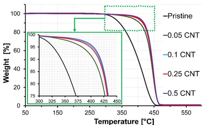
FIGURE 6 TGA curves of the pristine and nanocomposite fiber mats
