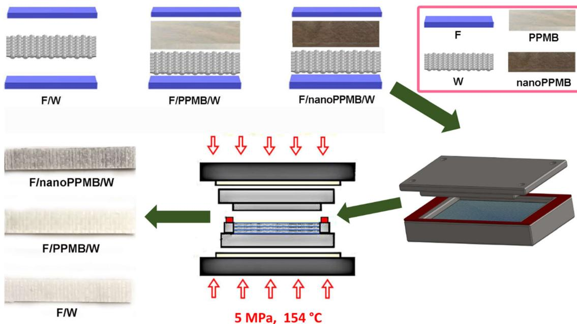
FIGURE 1 Schematic diagram of the SPC production process
